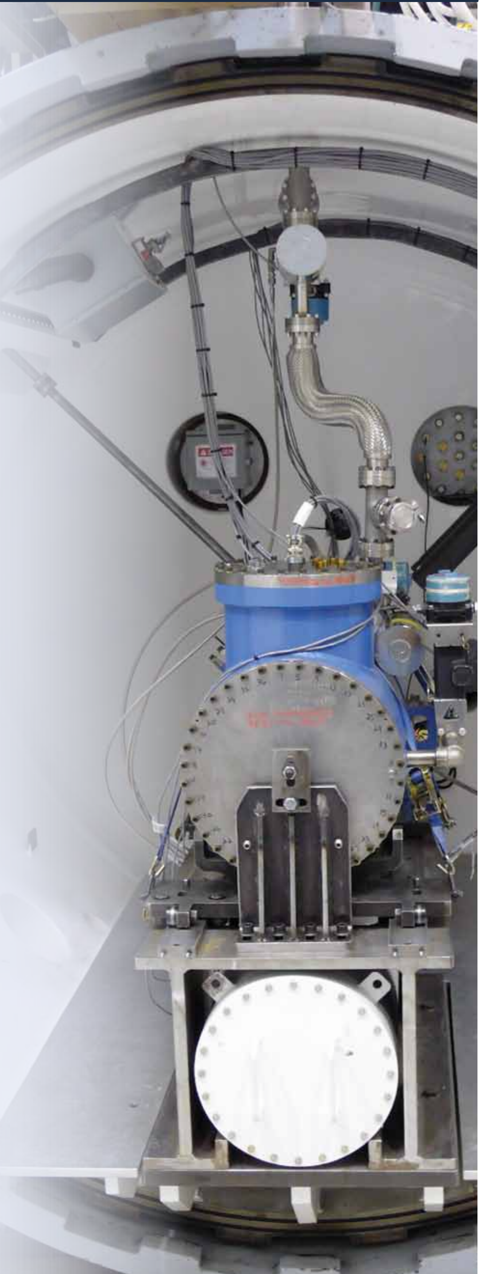
The above photo shows the Primary Target Chamber at the end of the JASPER gun barrel, inside of which a plutonium sample is shocked to high pressure to study materials properties.
