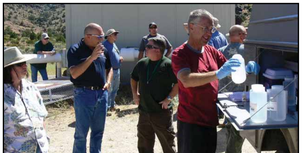
A groundwater specialist tests and seals RREMP well samples prior to transport.
