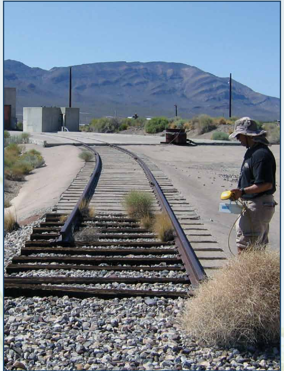
Worker conducts radiological survey on railroad tracks connecting historic nuclear rocket development facilities.
