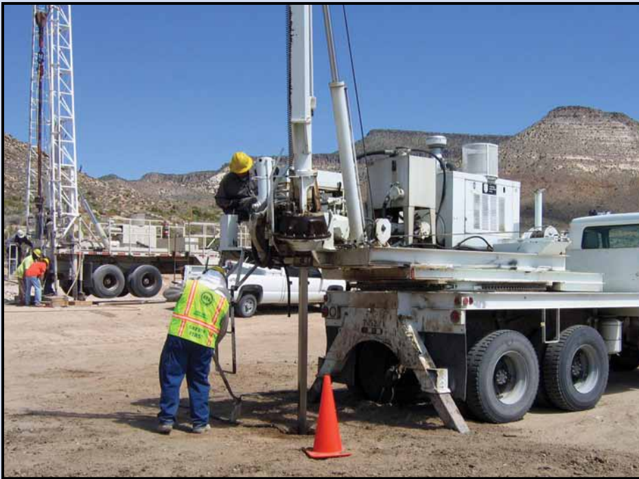
Workers break ground for an explosives hole test bed, drilling through a geology of mostly solid granite.
