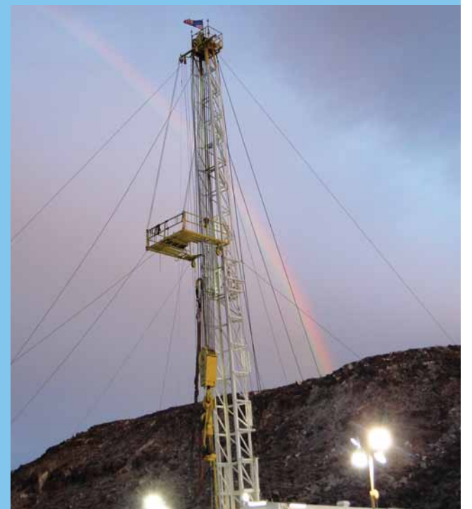
The new Pahute Mesa wells, designated ER-20-11 (bottom) and ER-EC-14 (above), were drilled to 3,003 and 2,378 feet, respectively. Depths of characterization wells typically range from 800 to 4,000 feet beneath the surface.
