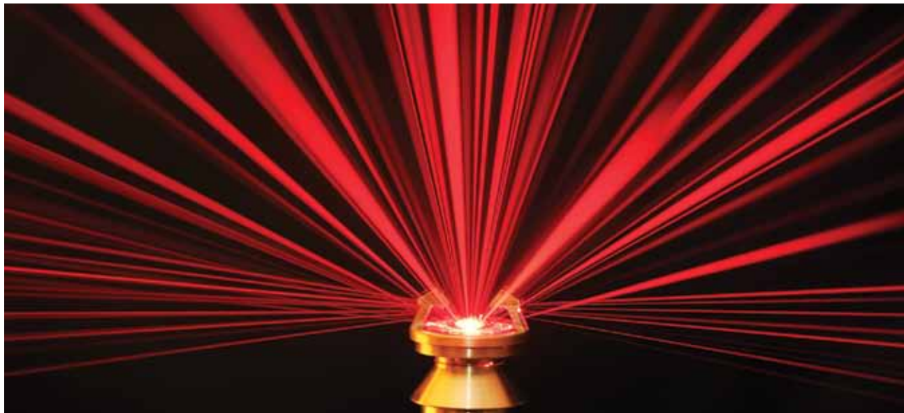
Gemini's advanced optical cavity probe design illustrates how a combination of lenses and mirrors can target hundreds of sampling points while materials are in motion. The "fisheye," or wide-angle, probe represents a "game changer" in the way scientists monitor the movement of an imploding surface.
