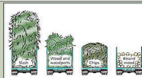
Volume differences of the same weight material by different product types Source: USDA Forest Service Forest Product Laboratory
