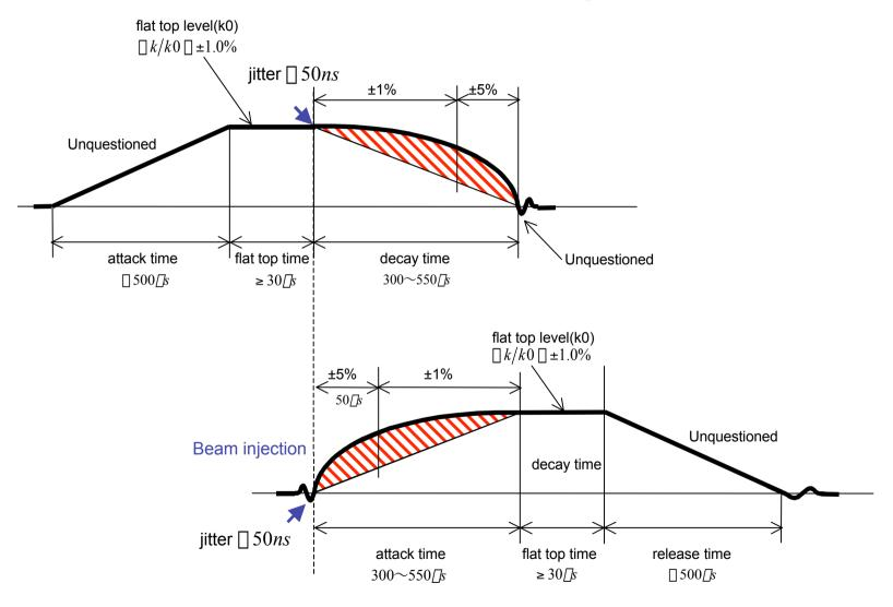
Fig.2 Current pattern of the power supply of the painting bump magnet in vertical
