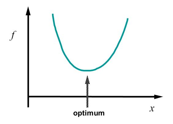
The optimum is where the gradient of the function is zero
