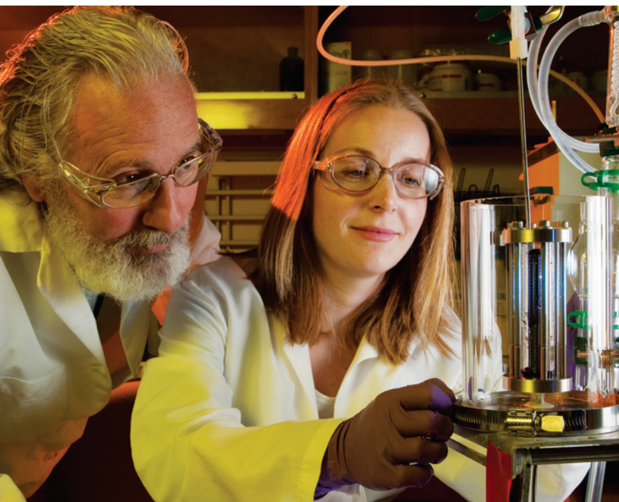
Chemists Roger Krueger (left) and Sarah Baker operate the wetted wall apparatus. This Livermore-designed test device measures the combined rates of all chemical and mass-transfer processes, including the concentration of CO 2 being vented.
