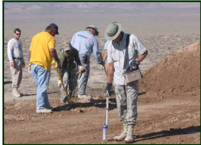
Unexploded ordnance (UXO) and radiation control technicians conduct a surface clearance survey at the TTR Bomblet Target Areas.
