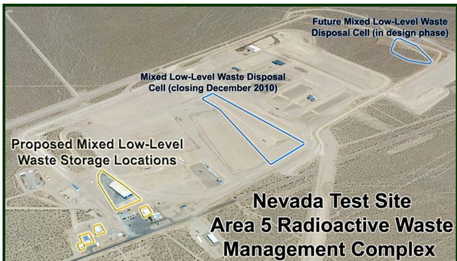
Proposed locations of mixed low-level waste storage prior to disposal in a RCRA-permitted disposal cell at the Nevada Test site Area 5 Radioactive Waste Management Complex.
