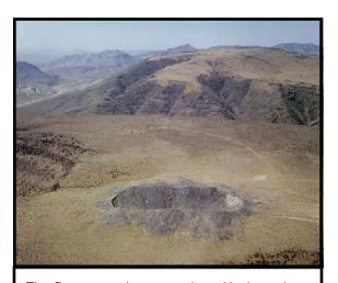
The *Buggy* experiment, conducted in the spring of 1968, was a series of five nuclear detonations used to produce a large trench. Buggy, along with several other tests, was part of the <a href="Plowshare Project">Plowshare Project</a> in which the U.S. government studied peaceful uses for nuclear weapons.
