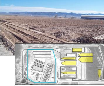
operate seven engineered, excavated cells for the disposal of containerized low-level and mixed low-level waste.
