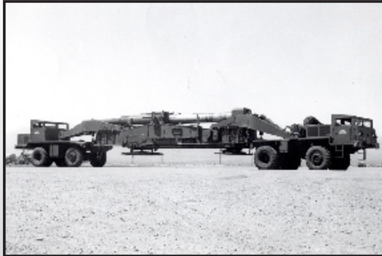
One of the 280 mm cannon's is shown completely assembled at Nellis Air Force Base on May 18, 1953, where it had just arrived by rail from Fort Sill, Oklahoma. Although it weighed 88 tons, its carriage was an ingenious foundation carried between two wheeled transporters, which were capable of speeds up to 40 miles per hour.
