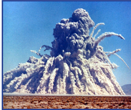
As part of the Plowshare Program, Sedan tested excavation capabilities of nuclear weapons for peaceful purposes.
