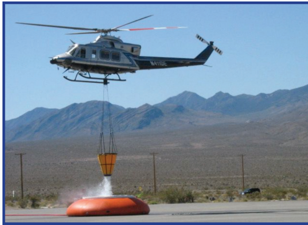
Energy II is utilizing one of the NNSS F&R portable water sources. These tanks, called "pumpkins" are placed in-service during a wildland operation by the fire prevention staff. F&R has two -3,000 gallon, two -5,000 gallon and one -10,000 gallon tank for immediate deployment.
