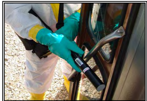
A responder checks for safe radiation levels in a bus after a simulated RDD attack on a metropolitan bus station.
