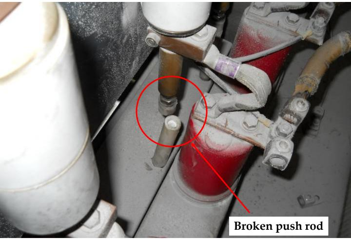
A recent electrical accident occurred when the control push rod for a vacuum bottle broke and allowed the contacts inside the bottle to close. In addition to the control push rod failure, a self-grounding mechanism in the disconnect switch had not been completely engaged. <u>The result of both failures was a</u> <u>miner receiving a severe electrical shock.</u>
