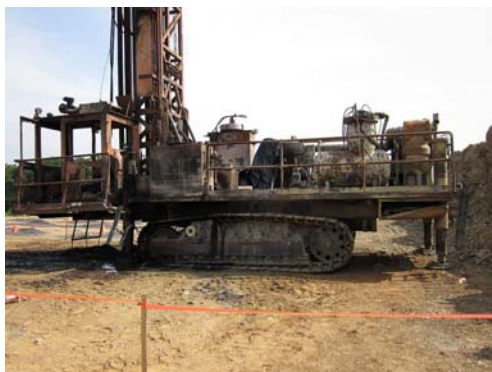
Drill rig after fueling fire
