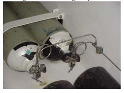
A dangerous condition can occur if the compressed oxygen system is damaged during movement of the refuge alternative. Sudden jerks, impacts, or improper handling may result in a leak in the compressed oxygen system. A slow leak can occur resulting in accumulations of oxygen. During the stress of a mine emergency, an improperly adjusted oxygen flow rate or unintentional damage to the system by miners can result in an oxygen enriched atmosphere inside of the refuge alternative. An
