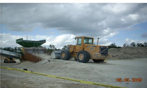
Victim exited front-end loader to check dump hopper. He was run over by the left rear tire.
