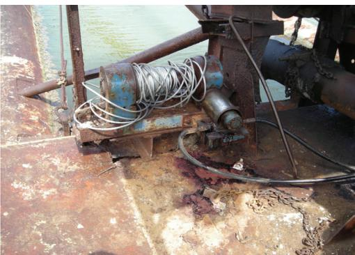
Victim's arm was pulled into a winch that was being used to position the dredge hose.
