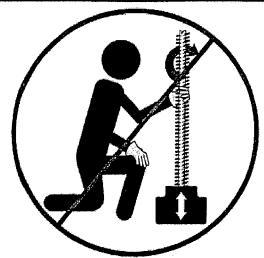
**NEVER** touch or hold onto a rotating drilling tool, wrench, or bolt.
