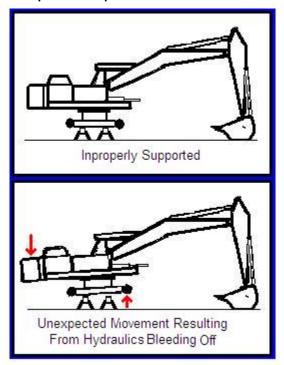
the bucket to the floor to provide stability. As the hydraulics bleed off, the bucket end (front) will in effect, transfer its weight to the counterweight (rear). This will reduce the weight on the front jacks or supports and place more weight on the rear ones. This redistribution of weight can cause the machine to twist or slide.
