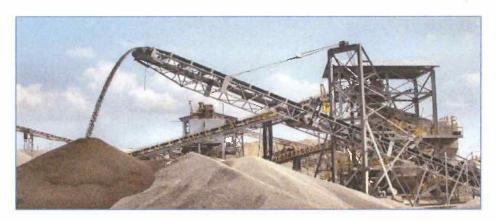
3 miners died in the last 20 months when the belt conveyor they were working on started unexpectedly, conveying them under obstructions or off the end of the belt. In each case, the conveyor drive motor was not deenergized, locked and tagged. In one accident a co-worker knew the victim had not locked out. Two of the victims had less than 6 months of experience.
