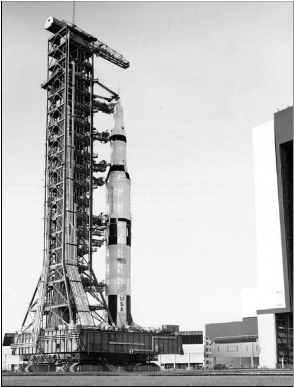
Figure 17. The Apollo Saturn V 500F Facilities Test Vehicle, after conducting the VAB stacking operations, rolls out of the VAB on its way to Pad 39A to perform crawler, Launch Umbilical Tower, and pad operations. (NASA Image Number 67-H-1187.)
