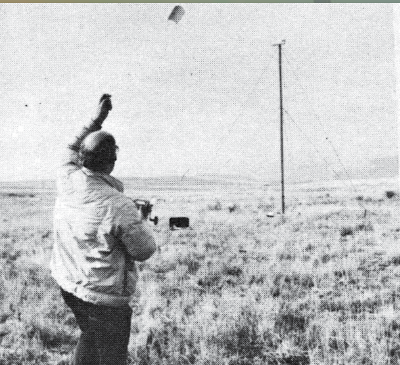
Researcher Bob Baker, an Oregon State University meteorologist, takes wind measurements in 1979. Pinpointing areas with the greatest wind potential was essential to siting generators for BPA's wind programs of the early 1980s.
