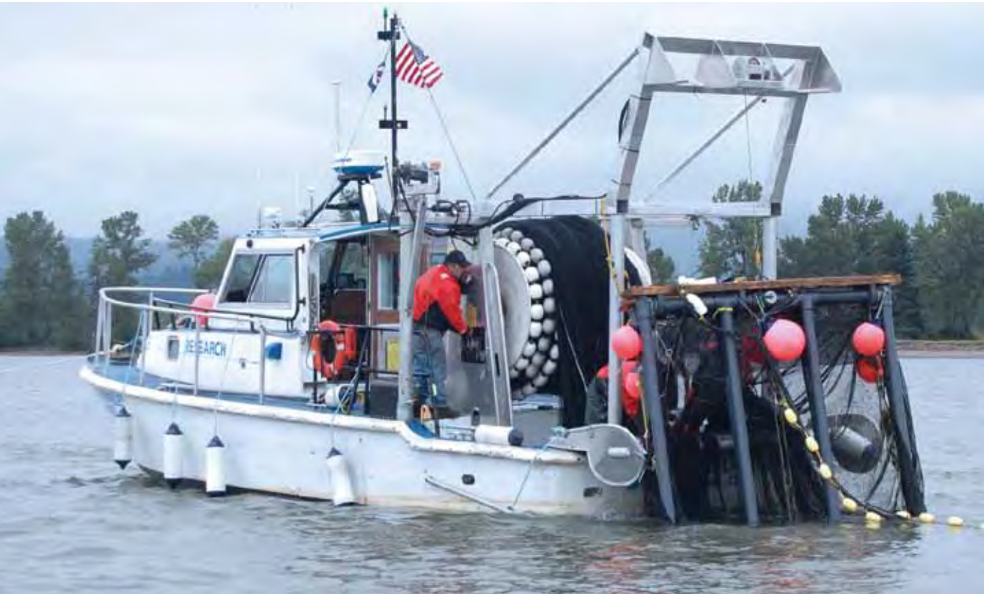
A NOAA Fisheries research vessel reels in a mobile PIT tag detector that captures data from tagged salmon and steelhead migrating to the ocean.
