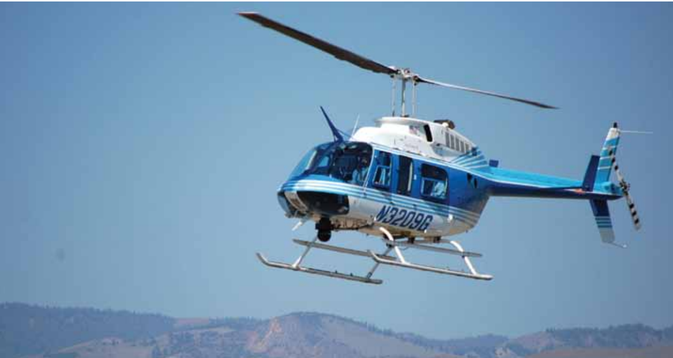
A BPA helicopter equipped with an infrared camera, typically used to search for hot spots on transmission lines, lifts off on a survey of Idaho rivers. The infrared camera revealed river temperatures that could help inform habitat restoration plans.
