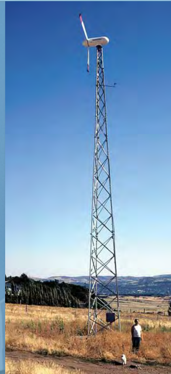
Recipients of BPA’s small wind generators were proud to participate in the program. This 2-kilowatt machine was installed near the Elmer Beeks residence in Murdock, Wash., across the Columbia River from The Dalles. (Rod Aho/BPA)
