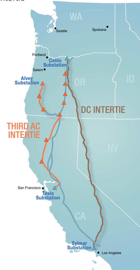
The Third AC Intertie, which includes components constructed by both Northwest and California utilities, appears in orange. It was energized in 1993, not long after utilities doubled the capacity of the DC line, which extends from The Dalles, Ore., to Los Angeles. Together, these transmission lines make up the largest single electricity link in the United States.
