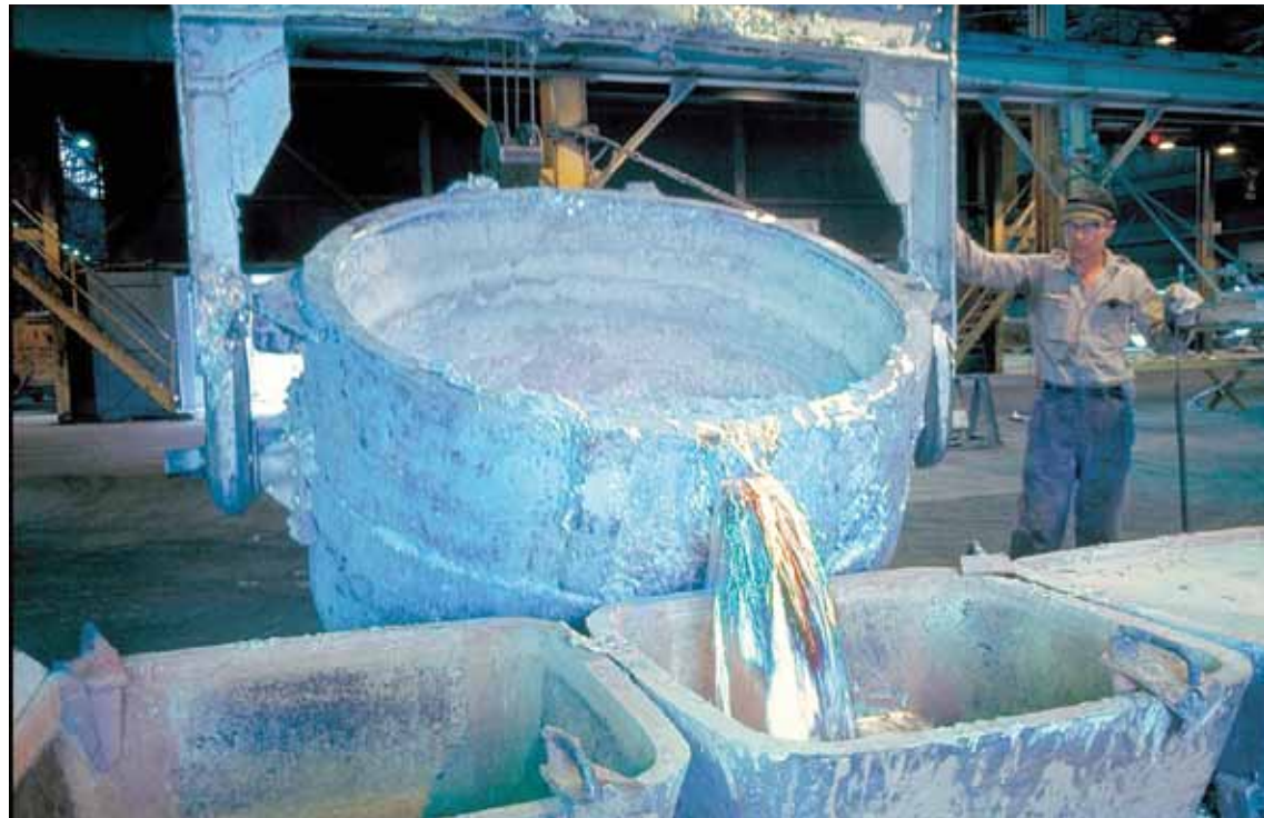
Molten aluminum poured into molds inside a smelter. Production of the metal requires vast amounts of electricity.
