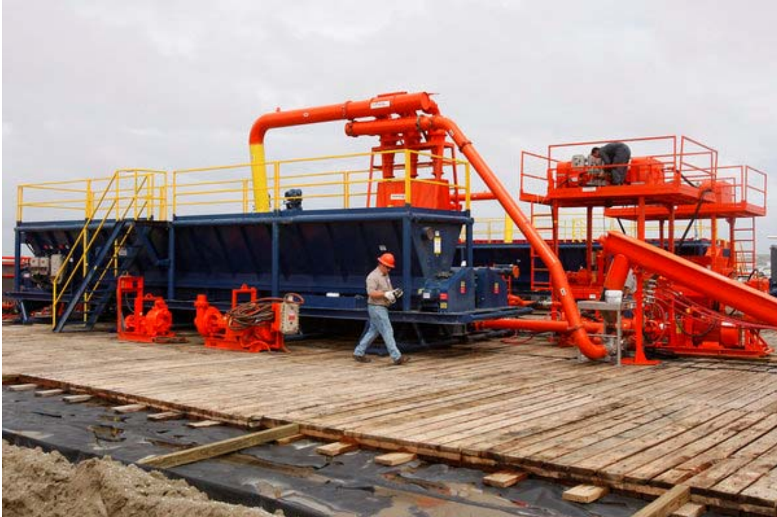
Figure 9. M1 SWACO Sand Treatment System (MSSTS) deployed at Grand Isle, Louisiana. Photo: from Associated Press.
