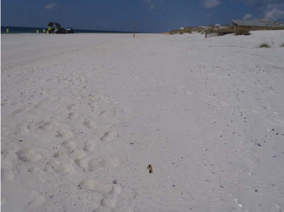
Figure 16. SCAT team photo of SRB cover on beach, estimated by SCAT personnel to be approximately 1%; image analysis determination of actual cover was 0.6%.
