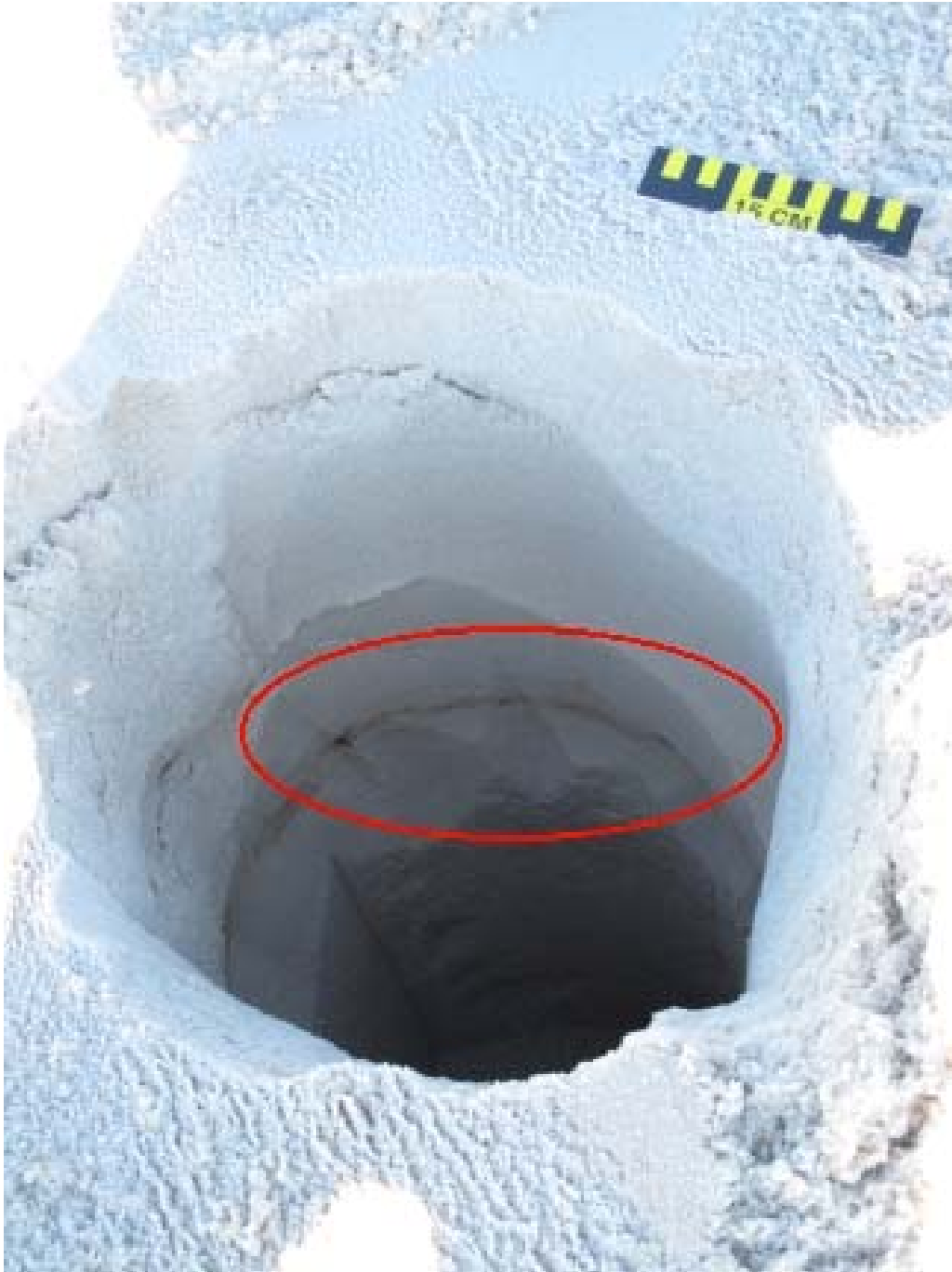
Figure 6. SCAT Team auger hole in the beach at Bon Secour National Wildlife Refuge, 8 January 2011. Buried oil layer circled in red.
