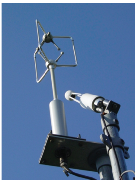
Figure 3: Eddy covariance system consisting of an ultrasonic anemometer and infrared gas analyzer (IRGA)
