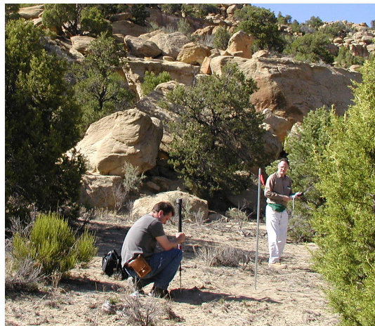
Soil-gas monitoring conducted by NETL personnel at an enhanced coalbed methane recovery site (Southwest Regional Sequestration Partnership) located at the San Juan Basin in northern New Mexico.
