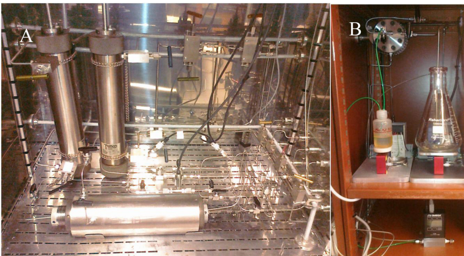
Figure 1. High pressure and high temperature fractured core flow apparatus developed for simulating sealing of fractures. A) The core holder and injection fluid accumulators are mounted inside a constant temperature air bath. B) Liquid and gas separation beaker and flow measurement devices are shown.
