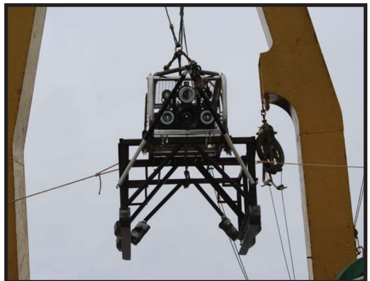
Figure 11.1. (A) The photographic/video imaging system, and (B) the addition of skis and supports to the body of the system that enabled consistency of altitude off the seabed (see Protocol Deviations section for more information).
