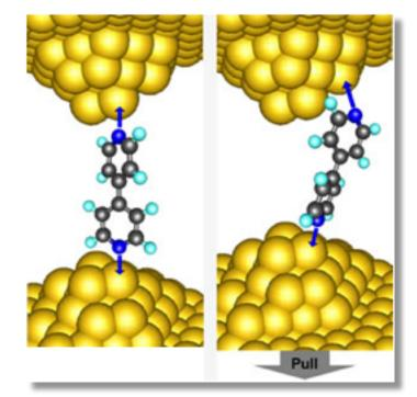
Schematics showing the molecular junction configurations for a model nanoswitch based on a junction between gold electrodes and a bipvridine molecule that is either vertical or tilted.
