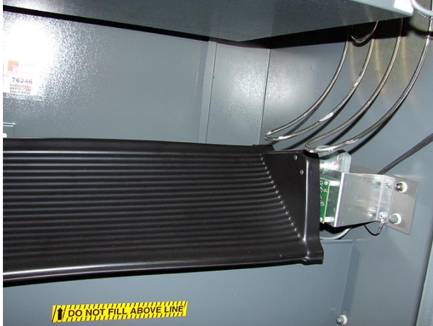
Photograph 8: DS200 metal ballot box with diverter (internal)
