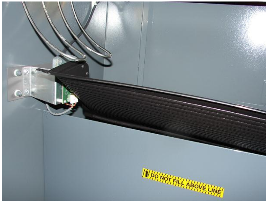
Photograph 9: DS200 metal ballot box with diverter (internal)
