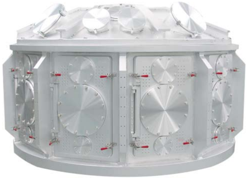
Titan’s long-pulse beam can be directed into the 2.5-meter-diameter target chamber through different ports. The short-pulse beam is directed through a dedicated port.
