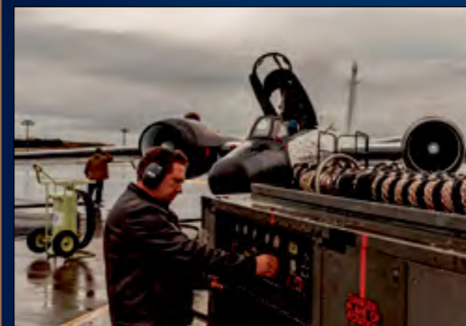
Francisco Augusto, 65th Operations Support Squadron Aerospace Ground Equipment, checks the Dash 60 Generator power output for the WB-57F Canberra while providing airplane power support Dec. 3. (Photos by Lucas Silva)
