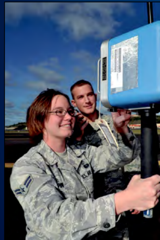
Airman 1st Class Ashley Stupin measures the properties of the radiation pattern from the glideslopes while Airman 1st Class Marcus Dennin calls in the readings during their ground checks, Nov. 7, 2012, Lajes Field. Both Airmen are airfield systems technicians assigned to the 65th Communications Squadron. (U.S. Air Force photo by Tech. Sgt. Chenzira Mallory)
