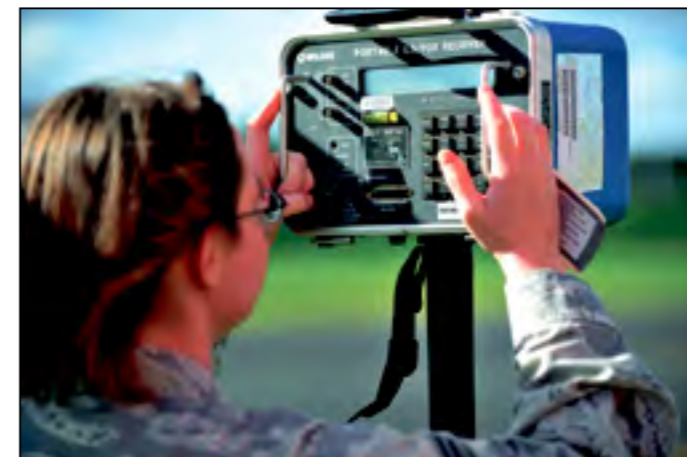
Airman 1st Class Ashley Stupin, 65th Communications Squadron airfield systems technician, prepares a portable instrument landing system receiver to conduct ground checks on the glideslopes, Nov. 7, 2012, Lajes Field. Stupin is using the receiver to measure the properties of the radiation pattern from the glideslopes. (U.S. Air Force photo by Tech. Sgt. Chenzira Mallory)
