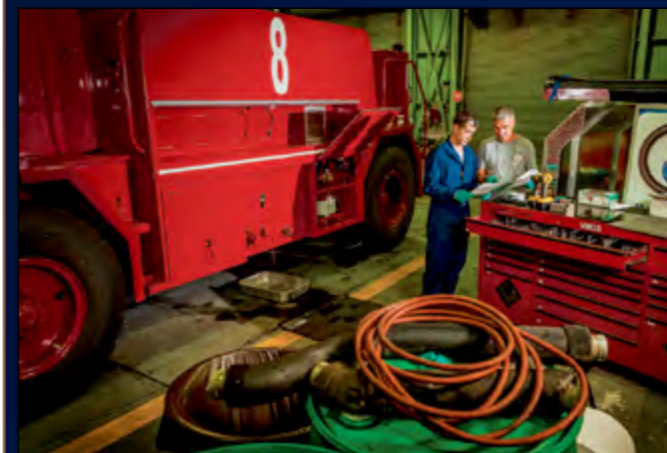
Ricardo Silva and Antonio Moniz, 65th Logistics Readiness Squadron, fire truck maintenance specialists, reference a Retrofit Kit Installation manual before installing a fill system on a 1986 P-19 fire truck, Sept. 10, 2012, Lajes Field. The fire truck maintenance crew upgraded the 65th Civil Engineering Squadron's crash response vehicles enabling the use of a 'no-foam' system. (Photo by Lucas Silva)
