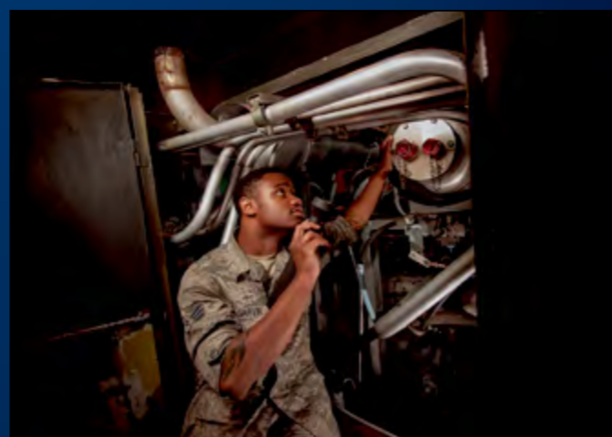
Senior Airman Diamonde Garvin, 65th Operations Support Squadron, Aerospace Ground Equipment journeyman, checks the tubing for leaks on a hydraulic test stand, Sept. 5, 2012, Lajes Field. The AGE shop provides, maintains and inspects equipment necessary to get transitioning aircraft to their destinations safely. (Photo by Lucas Silva)
