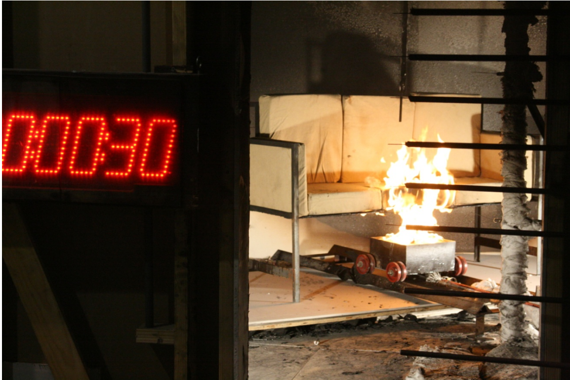
Figure 18. Large Flame Ignition Source Applied to Front Bottom (CF)
