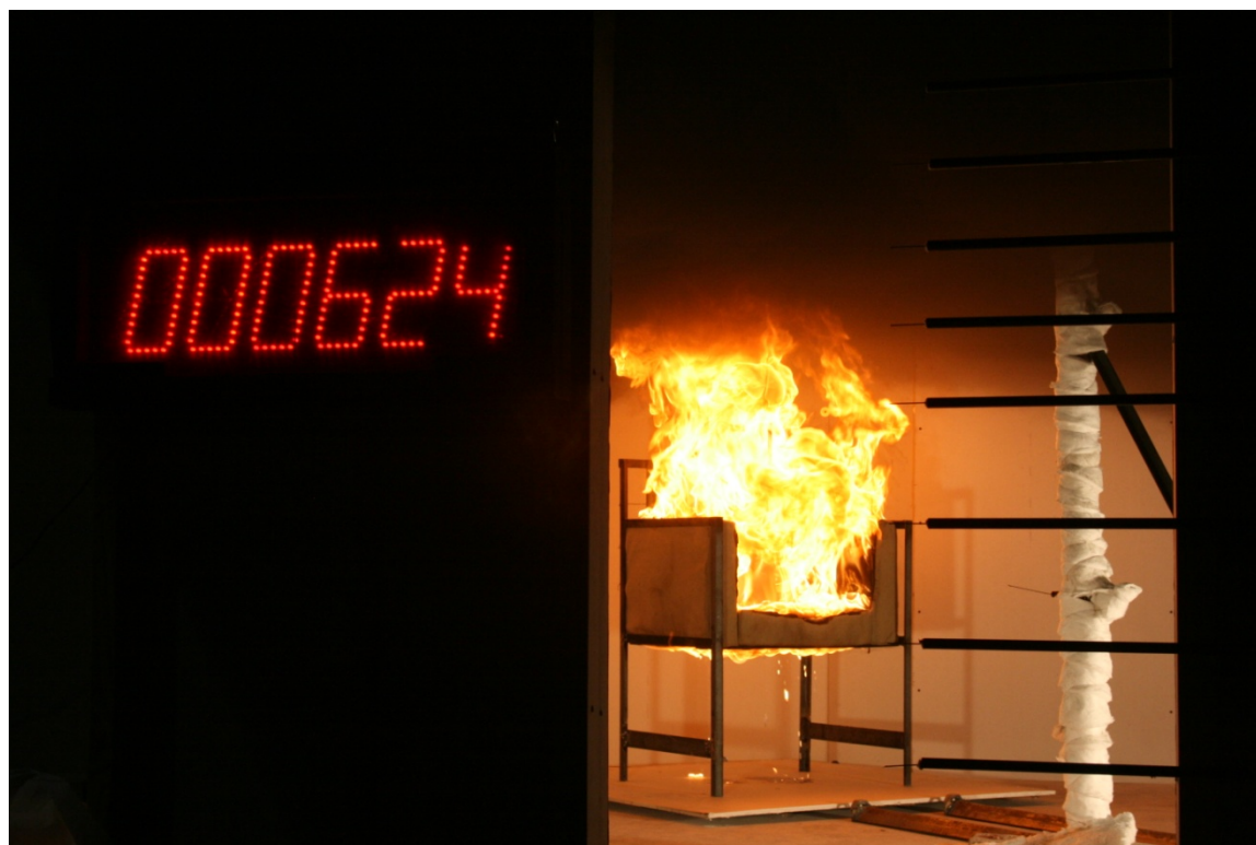
Figure 9. Test on 1-Seat Sofa near Peak Burning.
