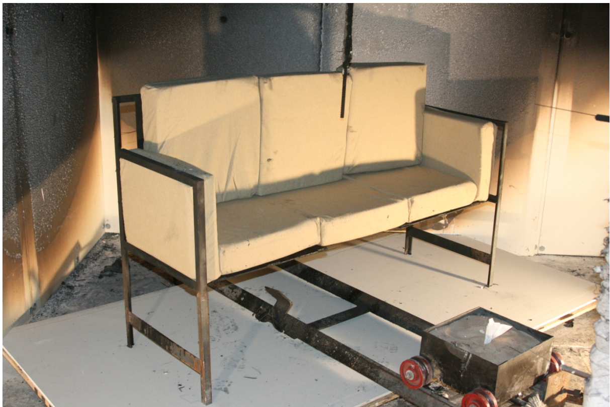
Figure 17. Front Bottom Large Flame Ignition Source prior to Ignition (CF).
