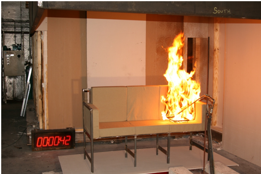
Figure 27. SOM123CS1 during Large Burner Flame Exposure.
