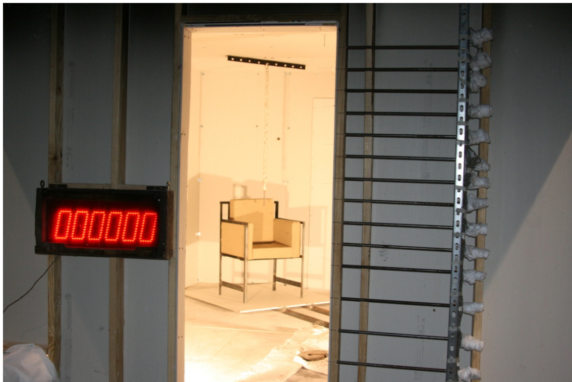
Figure 7. Doorway TC Tree Moved to the Side for Easy Room Access.
