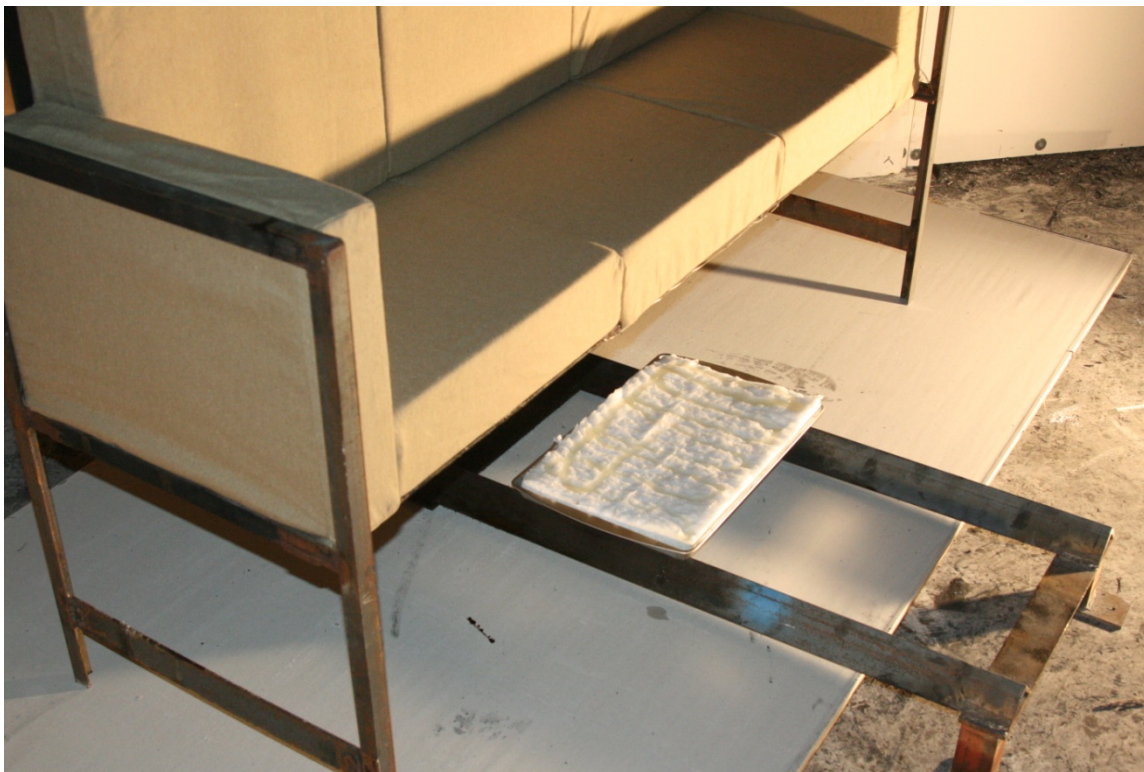
Figure 22. Gasoline Distributed over Ceramic Fiber Blanket (AF)
