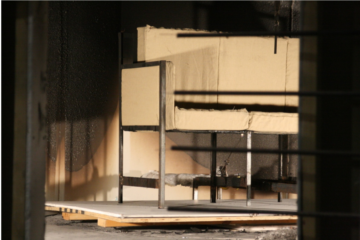
Figure 14. Small Flame Ignition Source Applied to Back (BB)
