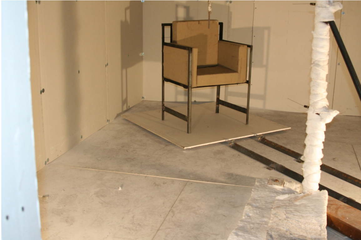
Figure 4. 1-Seat Sofa Mockup Placed on Scale prior to Testing.
