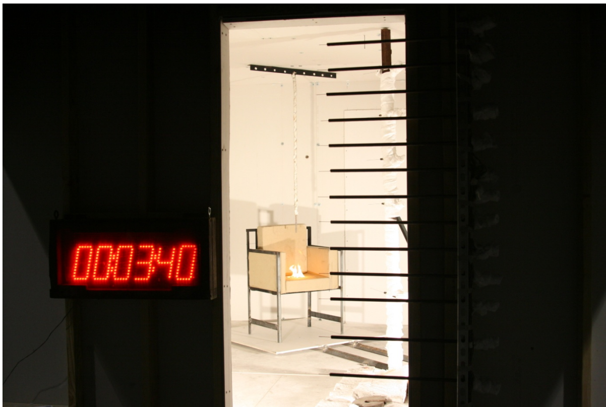
Figure 8. Test Shortly after Ignition with Small Flame.
