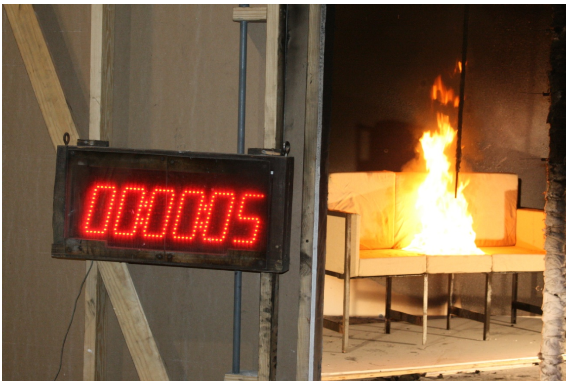
Figure 21. Liquid Pool Fire Applied to Top (AS).
