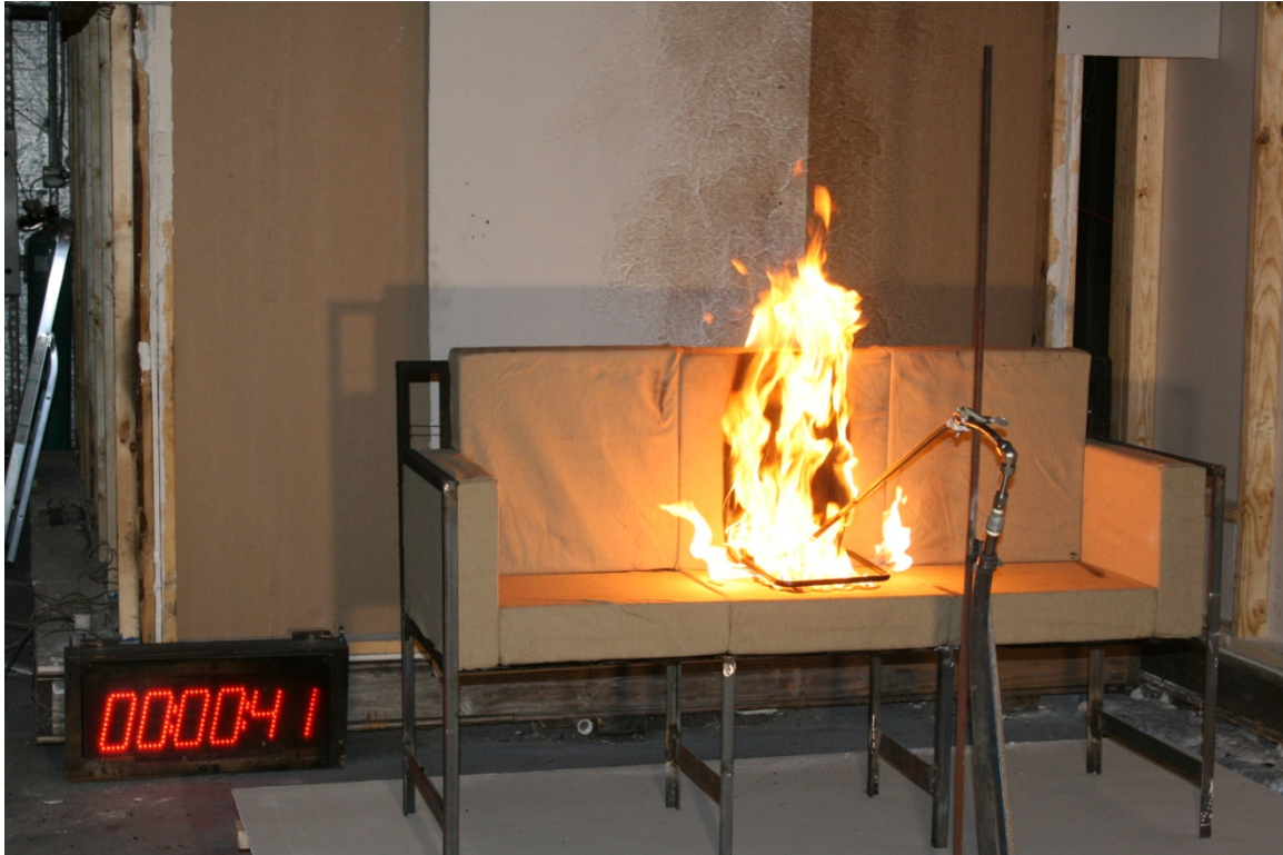
Figure 16. Large Flame Ignition Source Applied to Top (CS).
