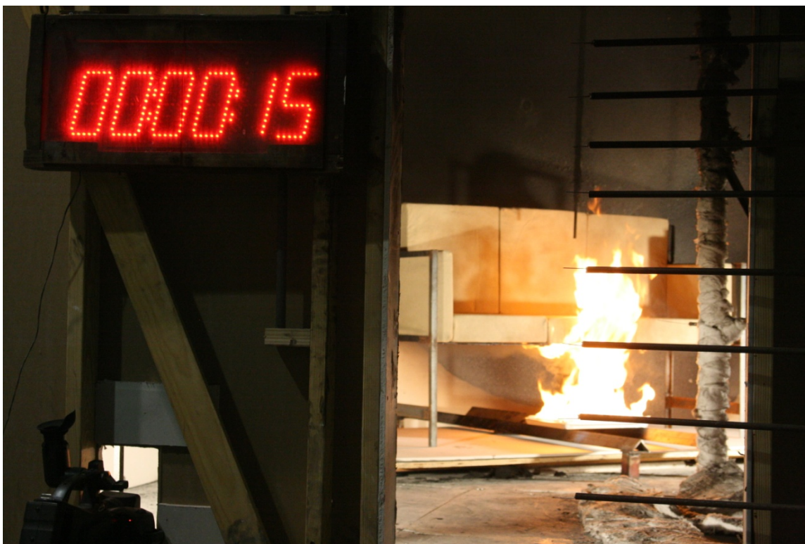
Figure 23. Liquid Pool Fire Applied to Front Bottom (AS).
