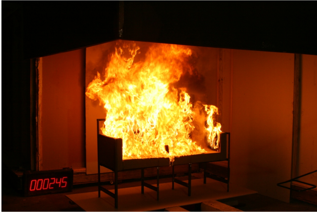
Figure 30. SOM123CS2: Flames Spread from Center to Both Sides.
