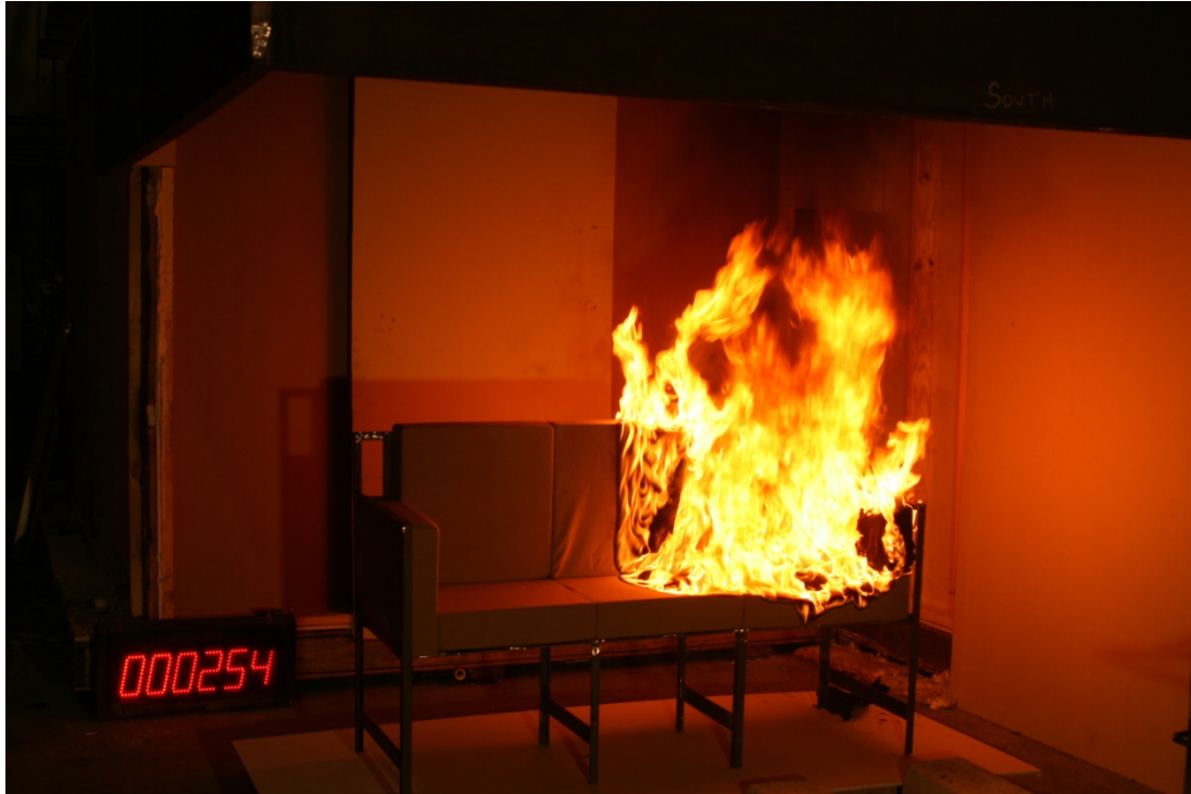
Figure 28. SOM123CS1: Flames Spread from Ignited Side to the Other Side.
