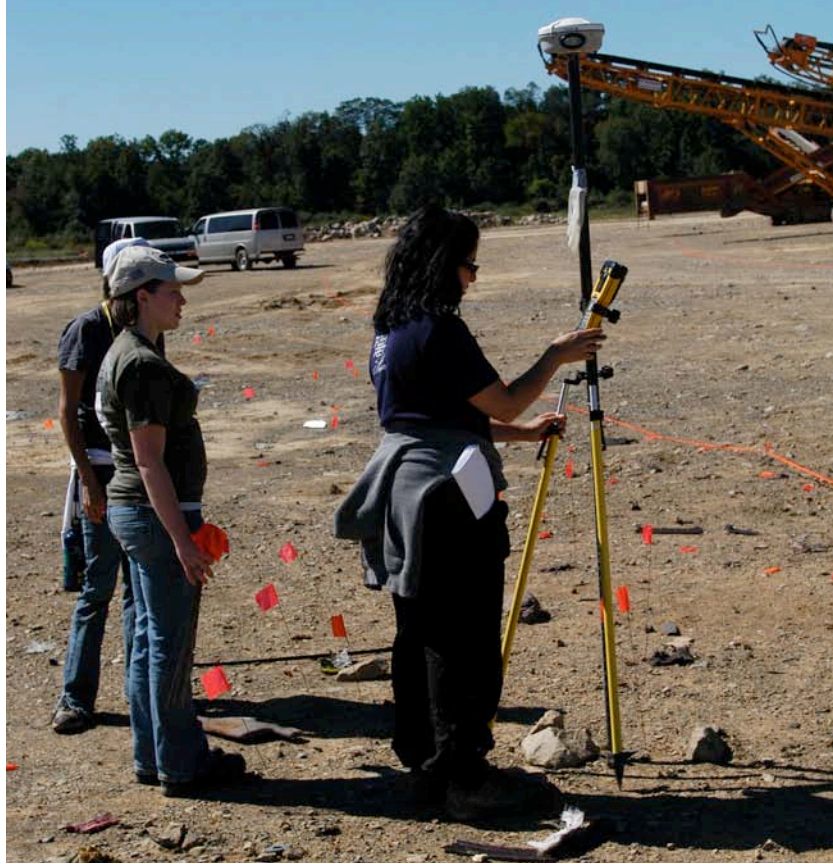
Figure III- 7. Team member using the R8 Survey Grade GNSS receiver to map corridors.
