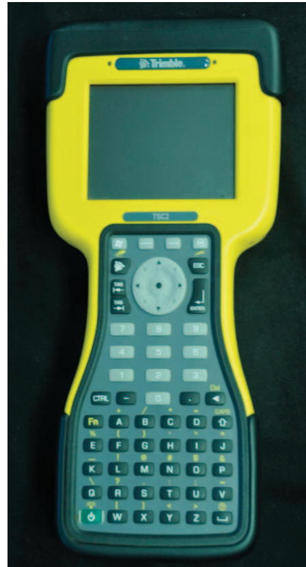
Figures II-10 and II-11. The Trimble R8 survey-grade GNSS (above) and Trimble TC2 handheld, ruggedized computer (right).
