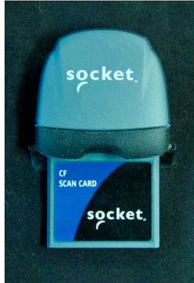
Figure II-5 .The Socket Type II CF Scan Card, which was fitted into the PDAs.
