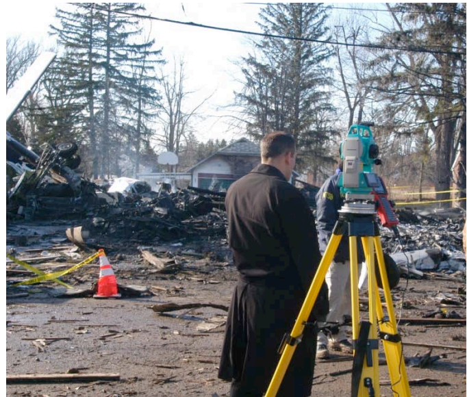
Figure 20 and 21. Establishing primary site datum (left). Total station assembled at the edge of the scene (right).
