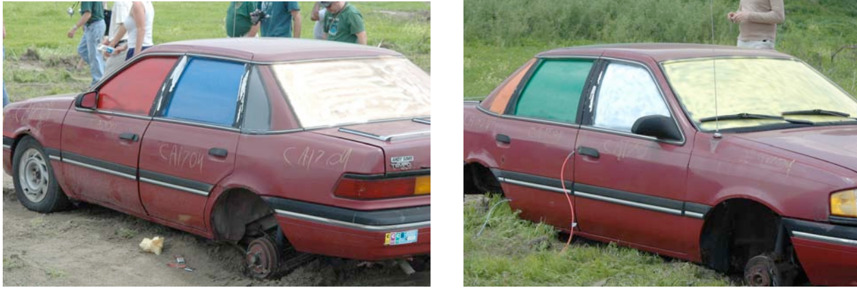
Figure III-2. Each window was spray painted in a different color to enable assessing the origin of glass fragments after the detonation.
