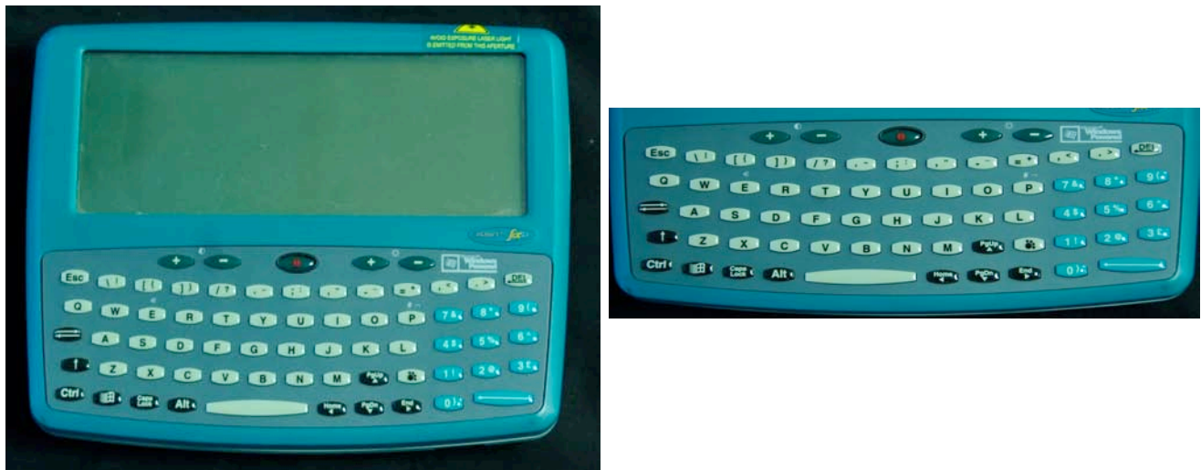
Figures II-2. The Huskey FexScan handheld barcode scanner with a full QWERTY keyboard.
