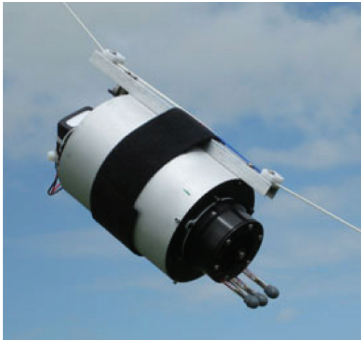
Figure 9. The Carousel, lifted by Apogee's Balloon, Carries Sorbent Tubes to Sample for Tracer Above the CO 2 Injection Area.
