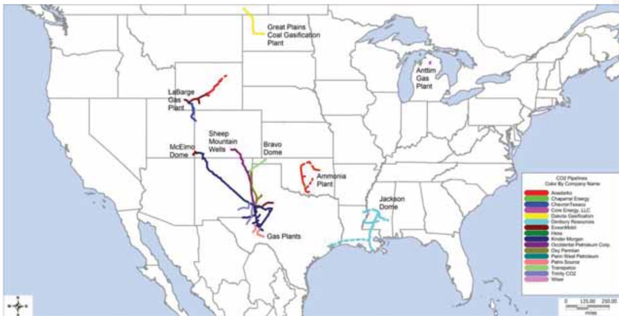
Figure 3-4. Current CO 2 Pipelines in the United States
