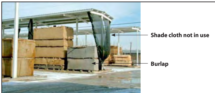
Figure 11-16. T sheds are used to protect lumber from the weather during air-drying. Lumber that surface checks easily, such as 8/4 oak, is wrapped in burlap or protected by shade cloth to slow the rate of surface drying during certain times of the year. Slower drying prevents surface checking.
