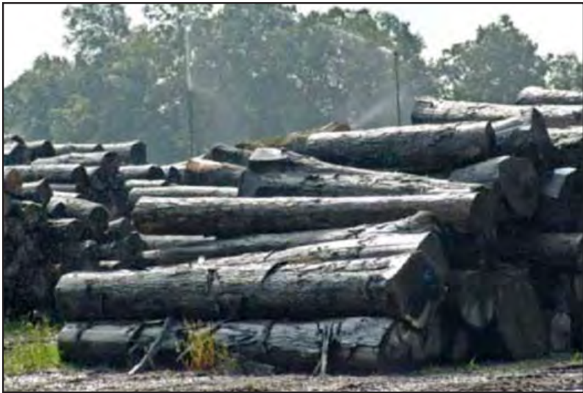
Figure 13-12. Water spray system for preventing log deterioration. Note the sprinkler heads in the background.
