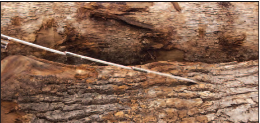
Figure 8-16. Bulges at the base of large white oak, also called “soda bottle effect,” are not considered defects.
