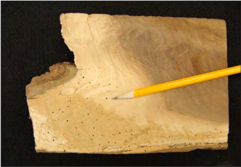
Figure 12-1. Powderpost beetle damage showing tiny insect exit holes (shot holes) in the sapwood of walnut. The sapwood of all species is susceptible to attack, although the heartwood of naturally durable species such as walnut and white oak is resistant.
