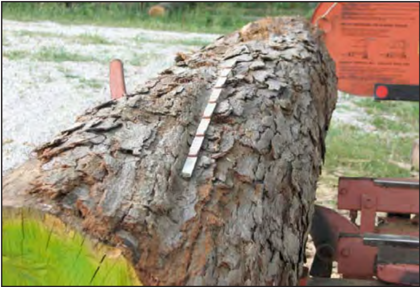
Figure 3-11. Spiral grain can be seen on this white oak log.
