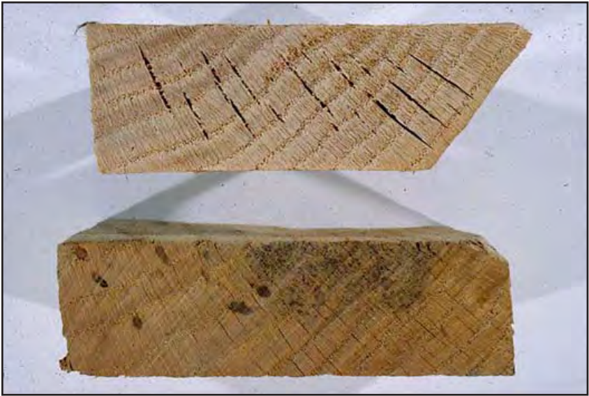
Figure 11-26. Internal checking or honeycomb in red oak. The checking was discovered after the top sample was cut from the board shown below.
