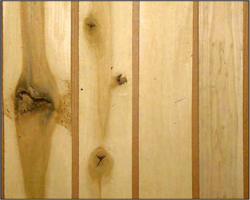
Figure 13-2. Range of color in yellow-poplar. The third piece from the left is about average for color in sapwood, while the fourth piece shows a very common gray or enzymatic stain.
