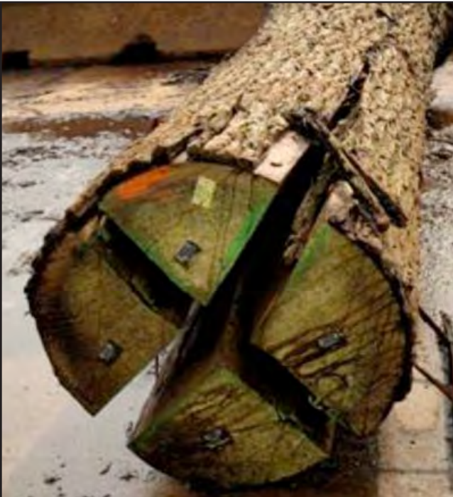
Figure 3-17. This high quality walnut veneer log has severely degraded due to the release of growth stress.
