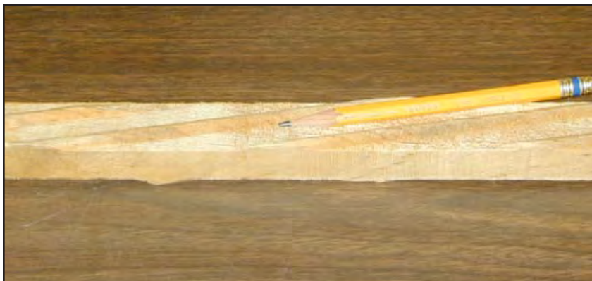
Figure 11-17. Drying stick or sticker with diagonal grooves, which help to prevent sticker stain or shadow on white woods.
