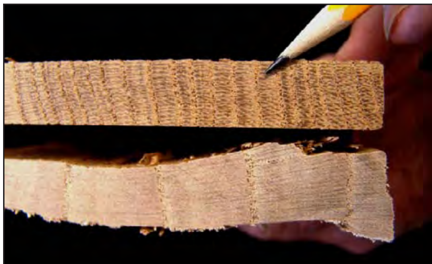
Figure 3-3. These two pieces of red oak are 5 to 5½ inches wide. The one on the bottom contains three complete and two partial rings. It is a fast-growing southern species called water oak. The top piece is average growth northern red oak and has 30 rings.
