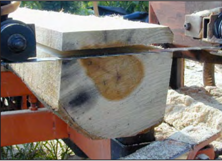
Figure 3-16. The release of growth stress resulted in a board that is bowed up towards the outside of the log and a work piece that is bowed down.
