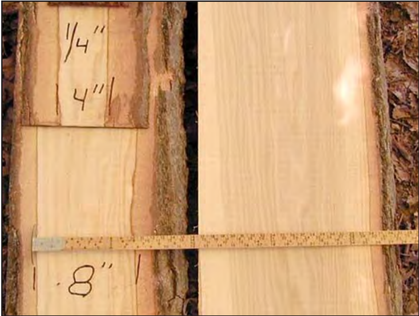
Figure 9-16. Care should be exercised in opening a log face. For this larger log, the sawyer opened the face to a narrow 4-inch width. The saw was lowered just \frac{1}{4} inch, in hope of getting a 6-inch wide face. Instead, an 8-inch wide face developed, resulting in wasted clear wood. The piece on the right shows the width that developed after the first board was removed.
