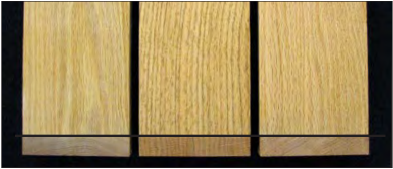
A. Ring porous red oak, shown in flat sawn (left), quarter sawn (center), and rift cut (right) boards.
