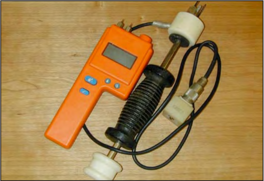
Figure 11-20. Electric resistance type moisture meter for estimating wood moisture content. The short prongs on the meter are for 4/4 stock, while the long needles can be hammered into thick stock.
