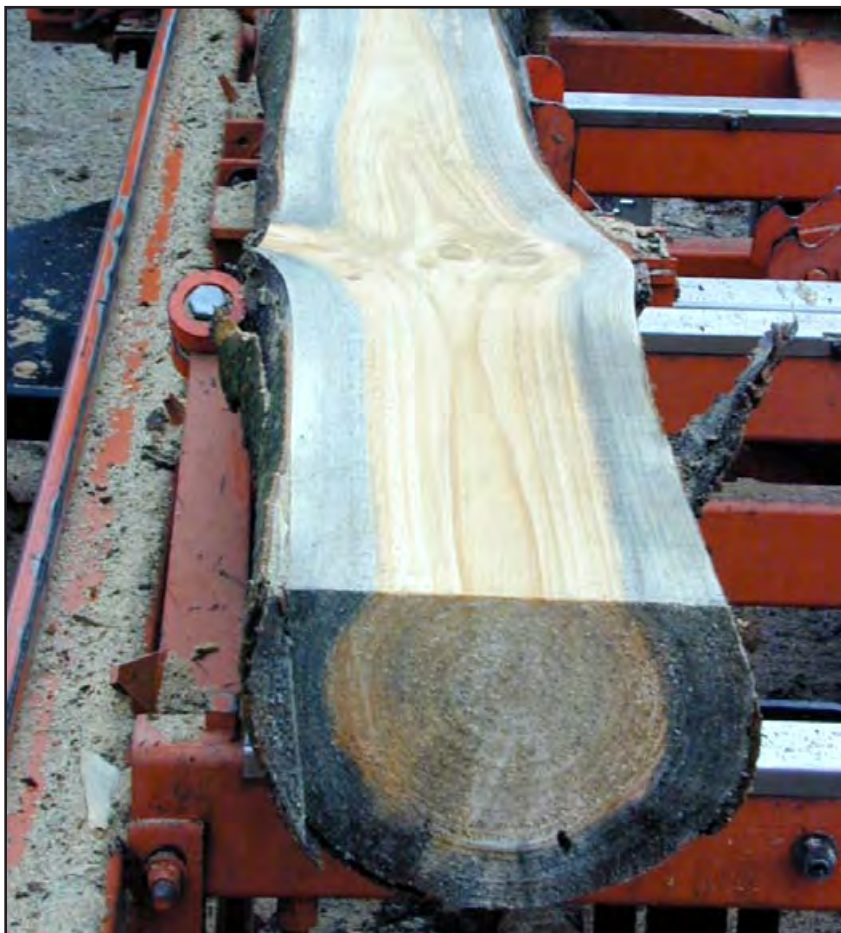
Figure 13-10. Blue stain or fungal stain in the sapwood of a white pine log.
