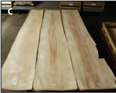
Figure 8-19. The end of a hard maple log shows a very small heartwood, which is desirable. The log end also shows two or more “black lines” or mineral streaks in the lower left quadrant. (B) These black lines result in streaks in the veneer. (C) The veneer from a different log shows the objectionable brown heartwood in contrast to the white sapwood.
