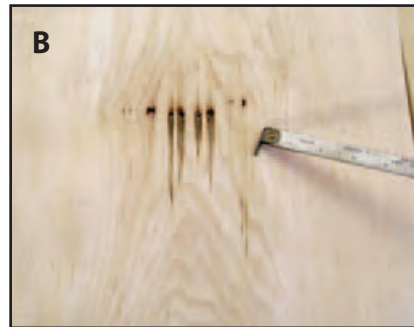
Figure 8-20. Bird peck forms a horizontal row on a hard maple tree (A), resulting in a defect in the veneer (B).
