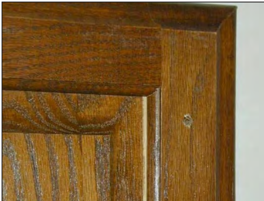
Figure 11-1. A raised panel kitchen cabinet door shows a white line on the right edge of the center panel due to shrinkage.
