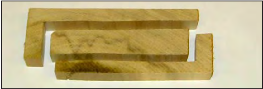
Figure 11-21. Crosscut samples for determining the moisture content of the shell and core of lumber. See Figure 11-23B for method of cutting samples.
