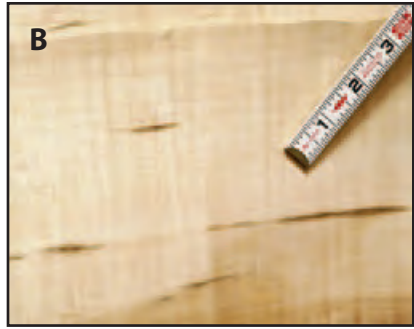
Figure 8-19. The end of a hard maple log shows a very small heartwood, which is desirable. The log end also shows two or more “black lines” or mineral streaks in the lower left quadrant. (B) These black lines result in streaks in the veneer. (C) The veneer from a different log shows the objectionable brown heartwood in contrast to the white sapwood.
