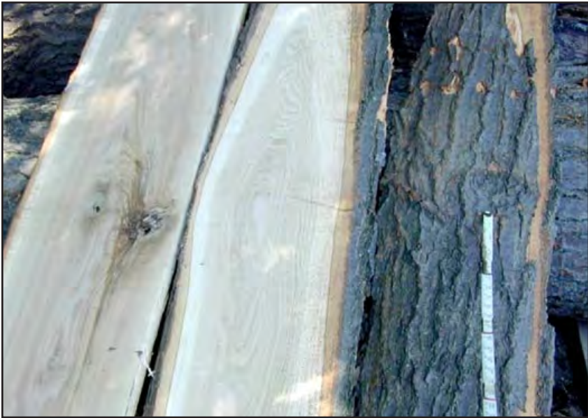
Figure 7-3. Overgrown knot in a red oak slab (right). The first board from beneath the slab is clear (center), but the back side of the second board shows a large defective area (left).
