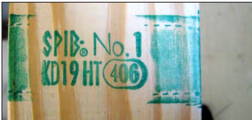
Figure 5-3. Example grade stamp showing Southern Pine Inspection Bureau (SPIB) as the agency, the grade as No. 1, kiln-dried (KD) to 19 percent moisture content, heat treated (HT), and producing mill number 406. The species is not given but implied, as SPIB deals exclusively with Southern Pine lumber.
