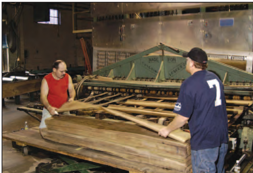
Figure 8-1. Veneer slicing operation showing the flitch or log half (back and right) being moved up and down against a stationary knife and the individual veneer sheets being stacked in the order that they are sliced.
