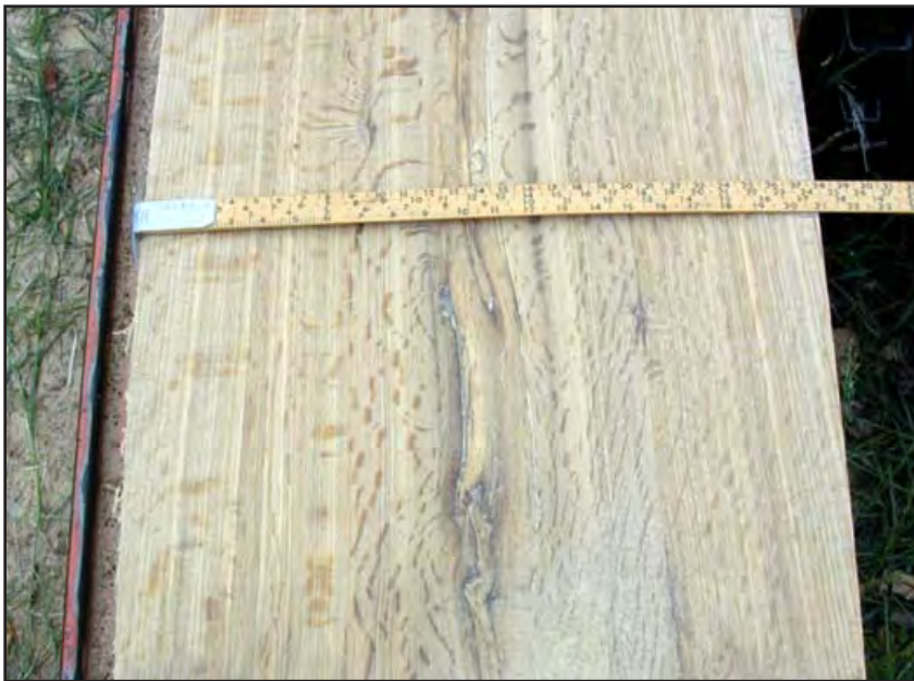
Figure 9-10. A wide board taken from near the center of a white oak log. Note the broad wood rays on the left (quartersawn). In the center of the board is a defective area from the heart of the log, which needs to be removed. The remaining piece on the right side of the board shows some fleck that disappears, resulting in a rift pattern on the far right edge of the piece.
