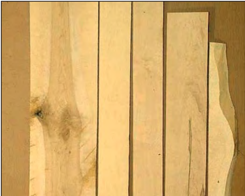
Figure 13-1. Range of color in hard maple. The board on the left shows both the dark heartwood and the preferred white sapwood. The four sapwood pieces on the right show a range of “white” in white hard maple lumber.
