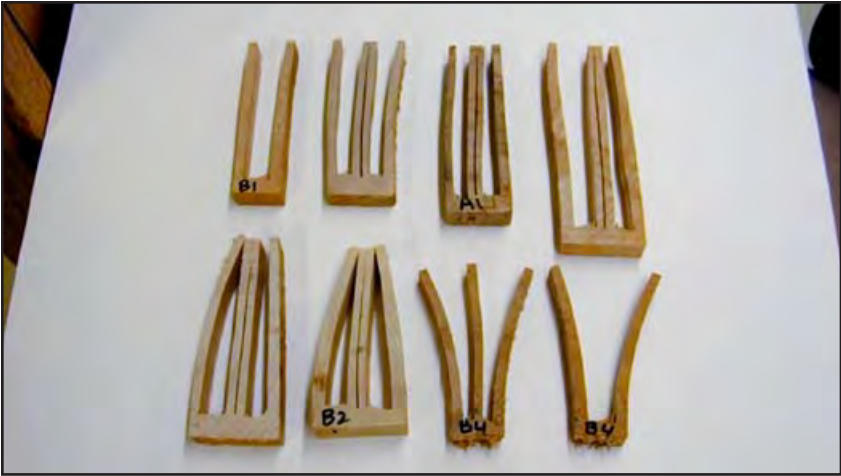
Figure 11-22. Stress or casehardening test in kiln-dried lumber. Prong tests in the top row show no stress. The two samples on the bottom left show casehardened lumber, while the two on the right show reverse casehardening.
