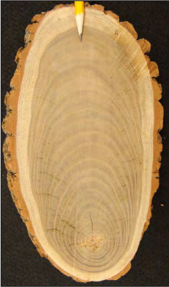
Figure 3-14. Tension wood is found in the upper side of leaning hardwood trees and branches. This is an extreme example.
