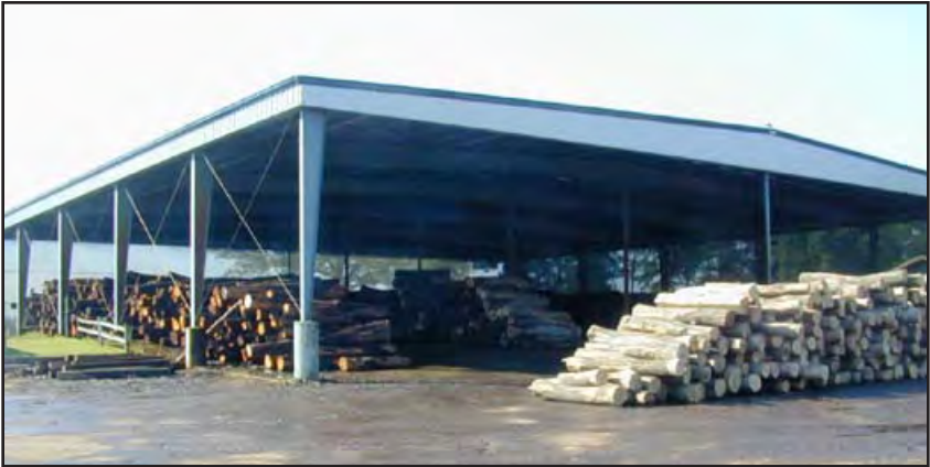
Figure 13-13. These high-valued logs are being protected by a water spray system. The shade from the roof slows the water evaporation rate and prevents the sun from heating the logs.
