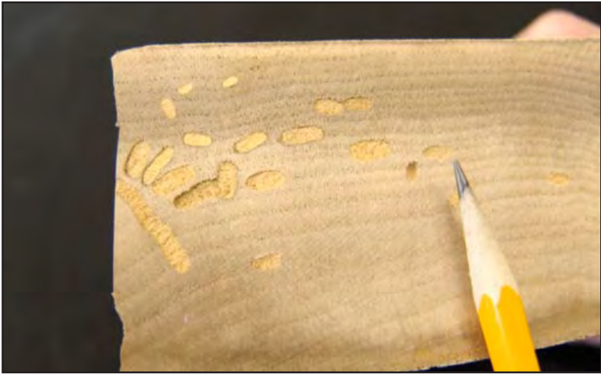
Figure 12-9. Flat-headed wood borer (Buprestid) damage in persimmon. Note the flattened oval shaped holes. Note also the cut tunnel (lower left) evidencing that the tunnels were in place before the wood was sawed.
