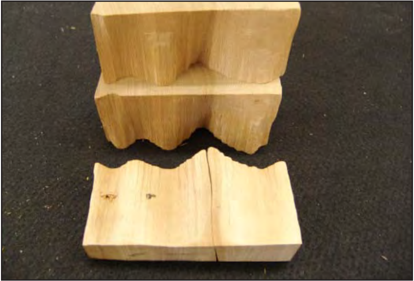
Figure 3-12. Interlocked grain in sweetgum. Note how the wood did not split uniformly but developed a wavy pattern.
