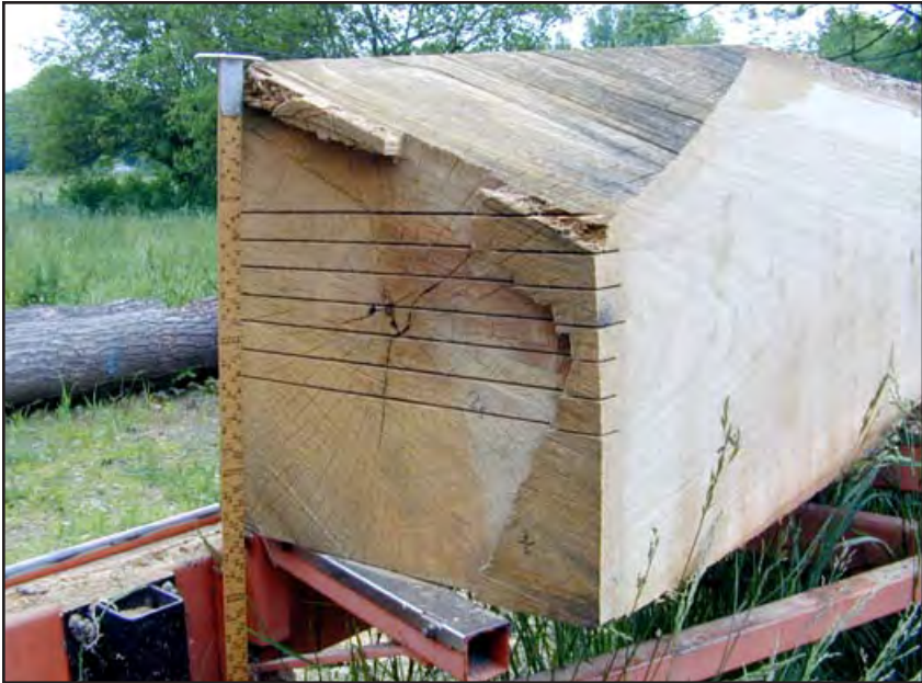
Figure 9-9. This quarter sawing method shows several pieces being taken out of the center of the log with a cant at the top and bottom. Note that the center saw line has been placed exactly on the pith. This maximizes figure or the amount of ray fleck and the number of pieces that can be removed before the boards are no longer considered quartered.
