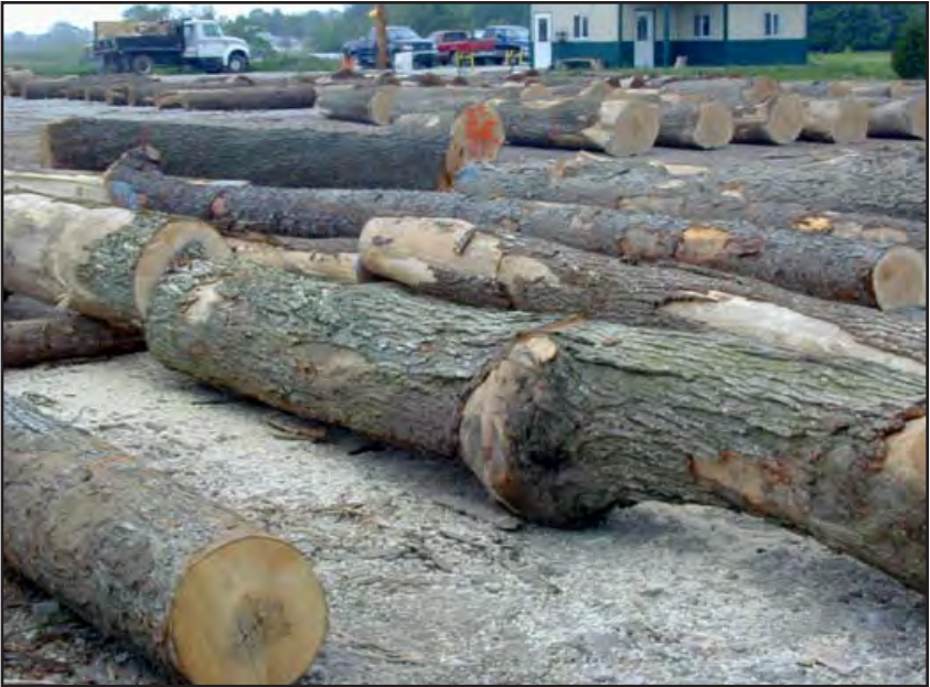
Figure 9-1. For these tree length stems, consideration must be given before bucking to producing relatively straight logs, with major defects positioned to maximize lumber grade yield.
