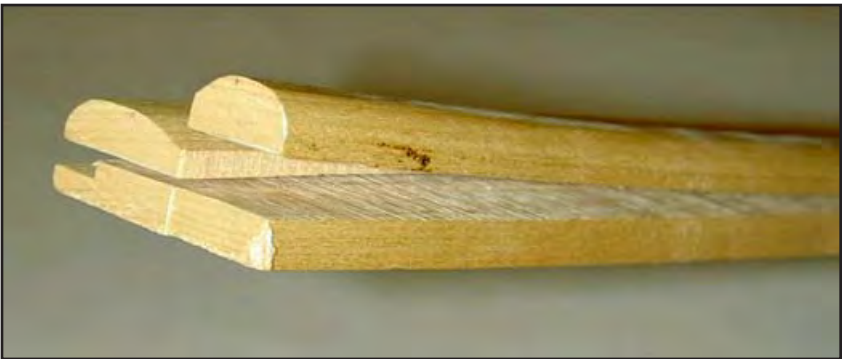
Figure 11-5. Casehardening or stress in the cabinet stile caused the entire door to warp. The stile was cut into sections so the amount of stress could be seen.
