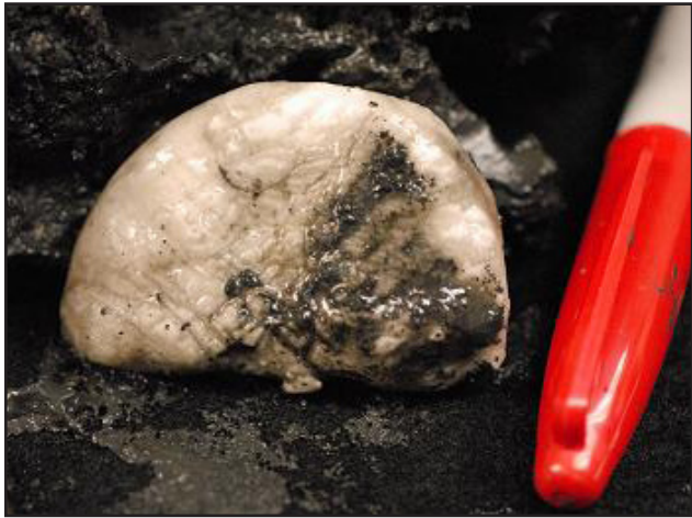
Example of nodular gas hydrate from zone of intensely deformed fine-grained sediments (courtesy NGHP Expedition 01, India)
