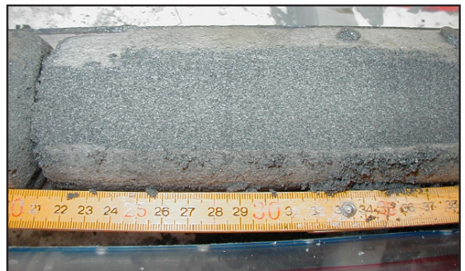
Example of disseminated gas hydrate (white specks) within porous and permeable marine sandstone from the Nankai Trough, offshore Japan (from Fujii, et al, 2005 ICGH Proceedings)
