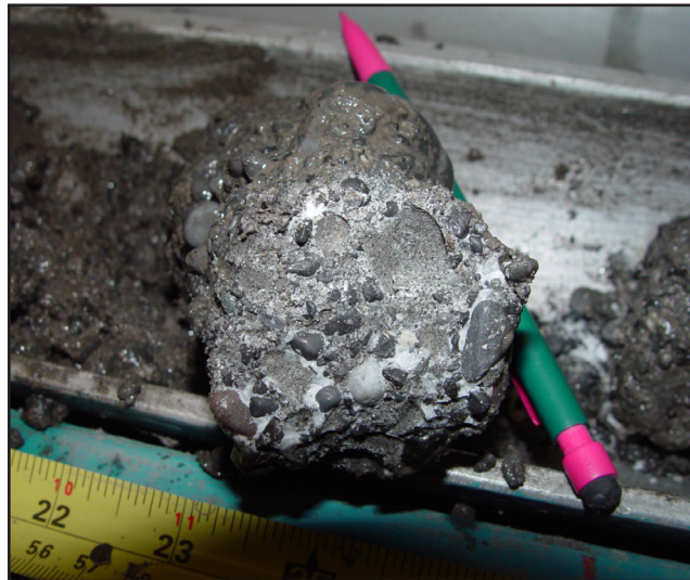
Example of disseminated gas hydrate (white) within porous and permeable Arctic sandstone from the Mallik site, Northwest Canada (courtesy Mallik 2002 Gas Hydrate Project)
