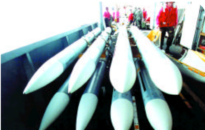
Advanced Medium-Range Air-to-Air missiles and AIM-7 "Sparrow" missiles are staged aboard the USS John F. Kennedy (CV 67) for quick loading on aircraft.
