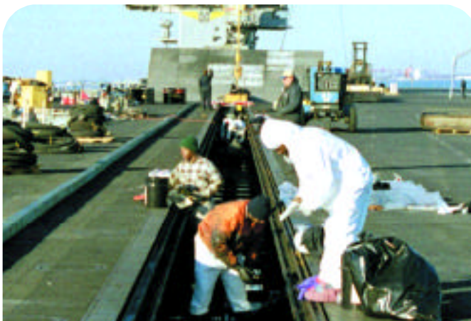
Shipyard workers work on catapult rods aboard USS Theodore Roosevelt (CVN 71).
