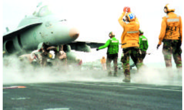
An Aviation Boatswain's Mate directs an F/A-18C "Hornet" towards the catapult on the flight deck of USS Enterprise.
