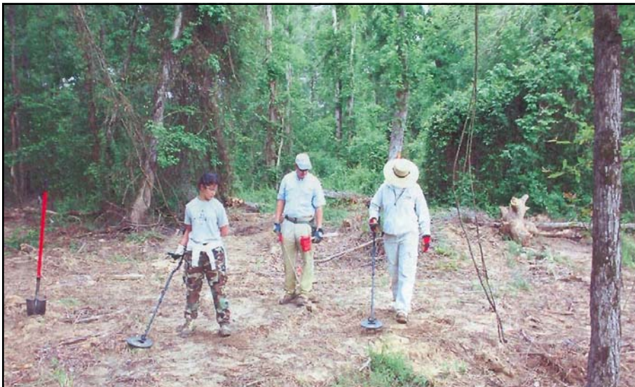
Instrument-assisted surveys help to identify the locations of spent munitions requiring removal from the Munitions Demolition Area (OD-33).
