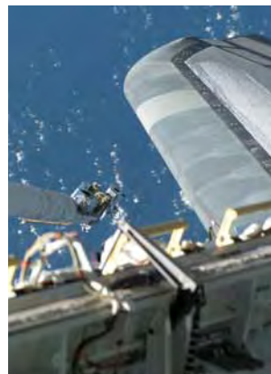
Sandia's orbiter inspection sensor housed in the payload bay, right, and being used to reach out toward the shuttle wing to scan tiles, left.
