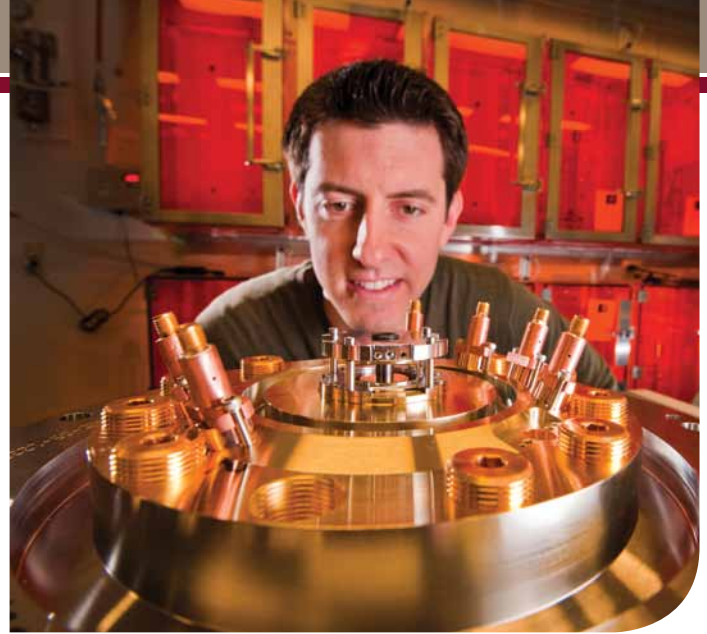
Physicist Ryan McBride pays close attention to the tiny central beryllium liner to be imploded by the powerful magnetic field of Sandia's Z machine. The larger cylinders forming a circle on the exterior of the base plate measure Z's load current by picking up the generated magnetic field.
