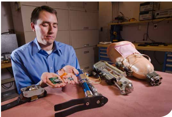
Steve Buerger displays implantable and wearable neural interface electronics developed by Sandia. He is part of a research team that is working on ways to improve amputees' control over prosthetics.
