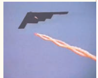
B-2 drop test involving B61 spin rocket motor
