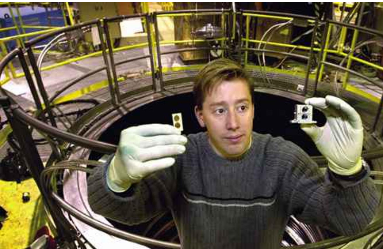
Sandia researcher Mark Knudson holds two flyer plates in his right hand and chambers of his high-tech gun in his left, used with the Z accelerator to launch dime-sized pellets to velocities exceeding 44,000 mph.
