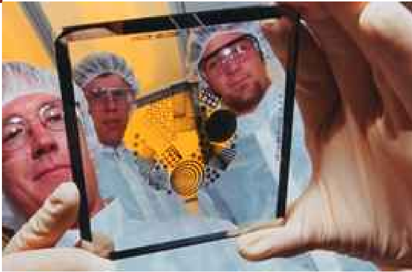
Sandians Doug Chinn, Craig Henderson, and Michael Winter display a chrome mask for LIGA, a three-stage production process for fabricating microscopic parts. (Courtesy of East Bay [Calif.] Business Times)
