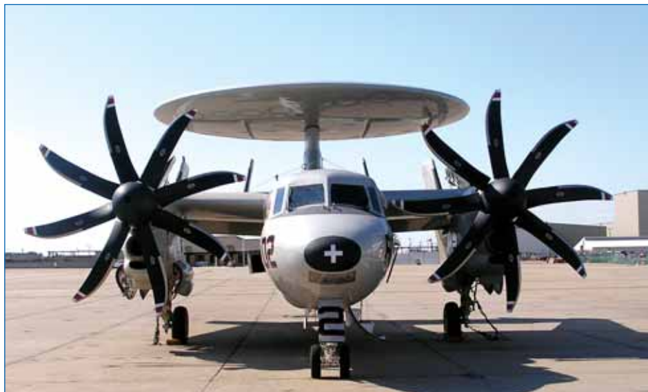
An E-2C+ Hawkeye increases performance and safety along with better maintenance techniques. Other improvements to the airframe include the Group II Mission Computer Replacement Program, which speeds up the Hawkeye's computers eight times faster than the older models.
